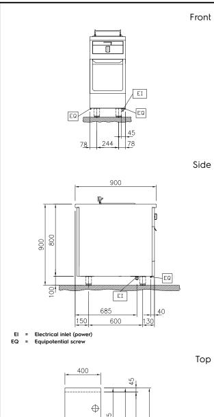
Electric Supply voltage: 400 V/3N ph/50/60 Hz Total Watts: 10 kW **Key Information:** Number of wells: Usable well dimensions (width): 240 mm Usable well dimensions 225 mm (height): Usable well dimensions 380 mm (depth): Well capacity: 12 lt MIN; 14 lt MAX Thermostat Range: 100 °C MIN; 180 °C MAX External dimensions, Width: 400 mm External dimensions, Depth: 900 mm External dimensions, Height: 800 mm Net weight: 75 kg On Base;One-Side Configuration: Operated
